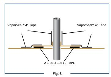
1.6. Holes or openings through VaporBlock® Plus™ are to be repaired by cutting a piece of VaporBlock® Plus™ 12" larger in all directions from the opening. Seal the patch to the barrier with 2-sided Raven Butyl Seal Tape and seal the edges of the patch with VaporBond Plus Tape.
