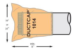
Styles 0610 & 1014 are manufactured from .002 mil. thickness orange polypropylene plastic with a 1/4" elastic band.
